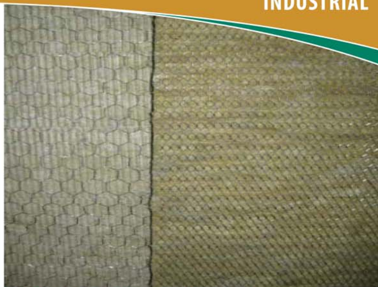
MPT® Metal Mesh Blanket OPERATING TEMPERATURE LIMIT: 1200°F(650°C)
